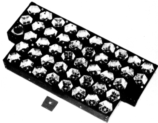
Fig. 35 - NTS-2 laser retroreflector
